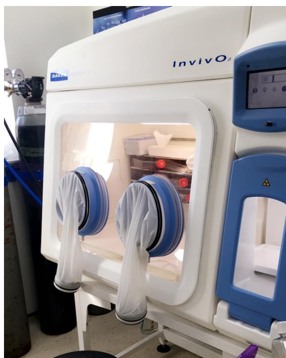
Figure 13: Image of InvivoO 2 hypoxic workstation used for growing UCMSCs
