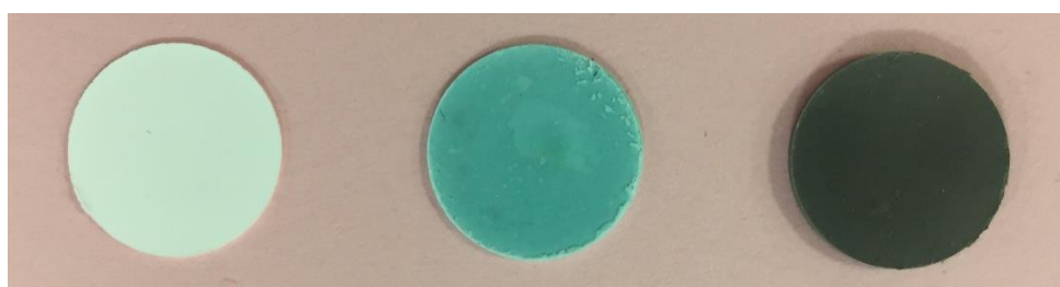
Figure 2.5. Zeolite samples pressed into pellets, parent zeolite MOR (left), copper impregnated zeolite before activation (middle), copper impregnated zeolite after activation (right).
