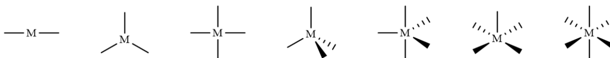
Figure 1.2. Common transition metal geometries, (from left to right) linear, trigonal planar, square planar, tetrahedral, trigonal bipyramidal, square-based pyramidal, octahedral.
