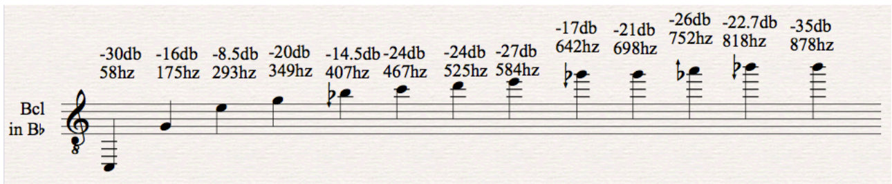
Figure 3.3.i: The most prominent partials on the bass clarinet's low C (sounding an interval of a 9th lower than written)
