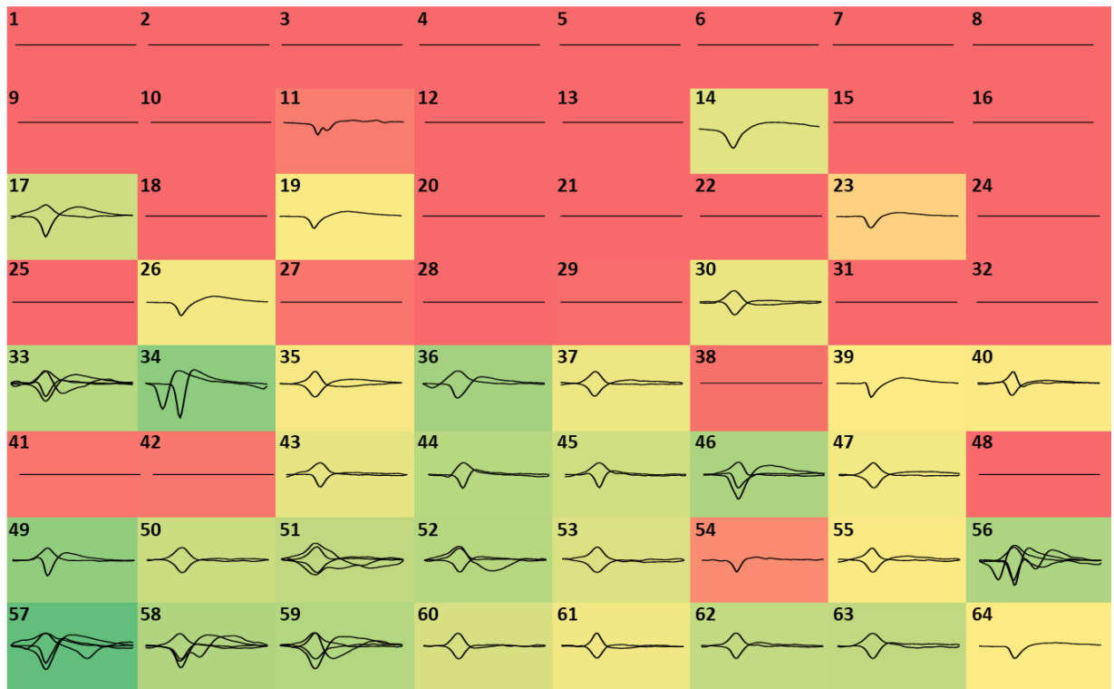
Figure 4.24: Centroid waveforms across a whole MEA, from CTX DIV 44, n=1. Each electrode was labelled from 1-64 and display the centroid(s) produced by that electrode. The same heatmap used in Fig.4.13 (CTX A DIV 44) was used as the background, with red-> yellow-> green indicating min (0), mean (524) and max (9551).
