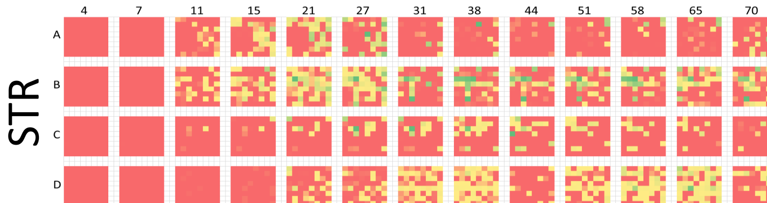
Figure 4.10: STR activity heatmaps. Each square is an 8 x 8 grid representing an MEA. Horizontal values 4-70 represent days in vitro (DIV) and A-D represent separate MEAs from repeat experiments. Red->yellow->green formatting indicates min->mean->max levels of spiking activity. Min, mean and max for each repeat as follows: A) 0, 137, 6002. B) 0, 661, 12064. C) 0, 126, 8610. D) 0, 199, 8705.
