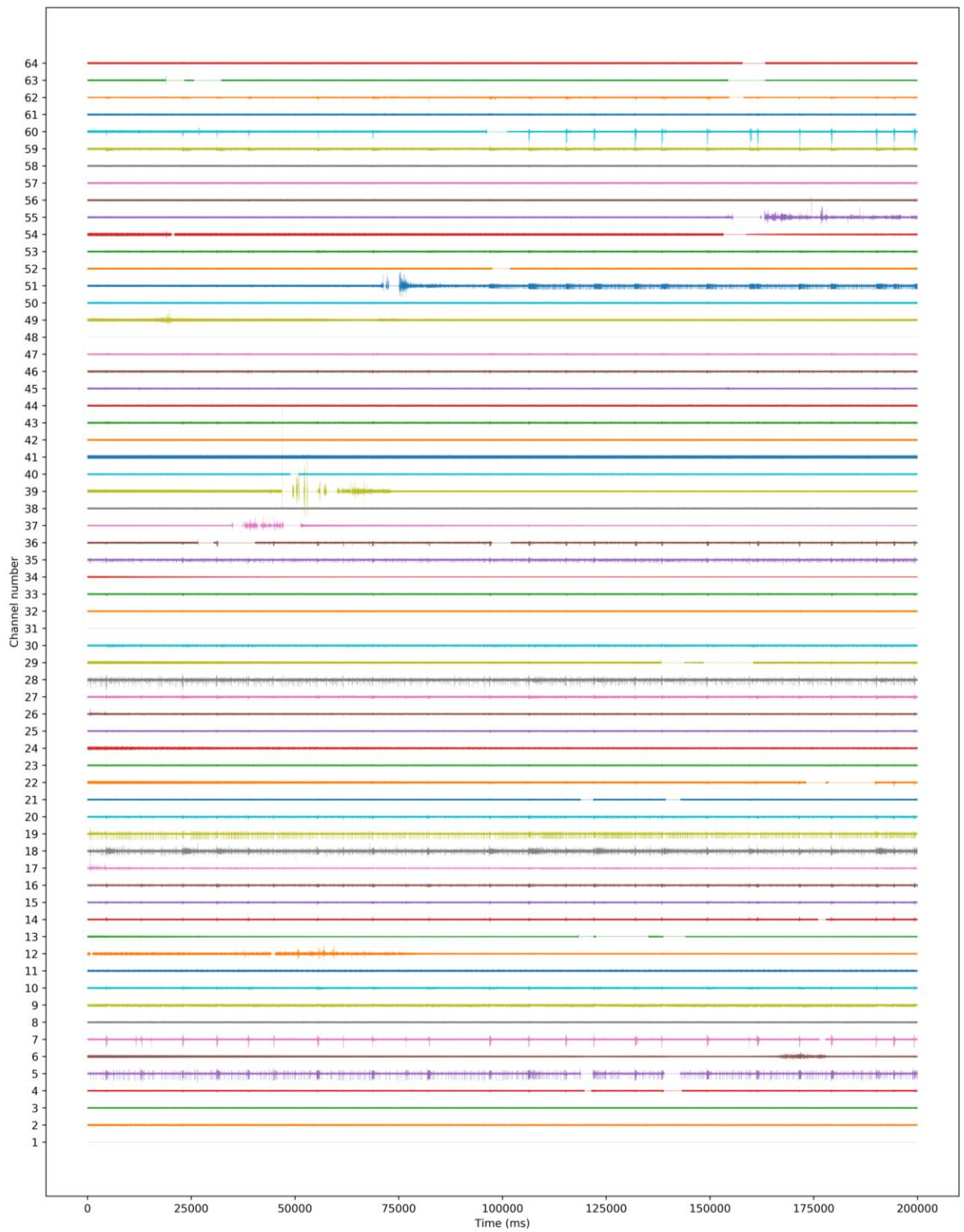
Appendix 2.4: 240 seconds of raw activity from all 64 electrodes of an MEA seeded with a STR neural culture, after 70 DIV.
