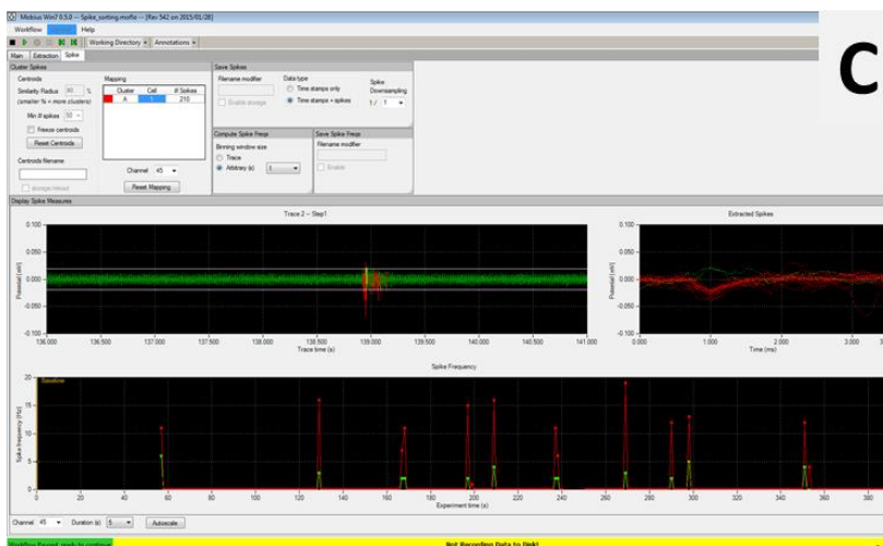
Figure 2.10: MOBIUS modules involved in the analysis process. The Spike_analysis/spike_sorting workflow is split into three main sections, A) MAIN, B) EXTRACTION and C/D) SPIKE. Each of these sections contains modules involved in the analysis of spontaneous extracellular activity from the MEA. Usage is detailed in text body.
