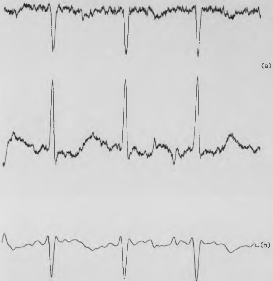
Figure 7.12 The result of applying high pass filter to remove dc and baseline fluctuations and then applying the adaptive technique to remove the skeletal muscle activity, the figure shows:
