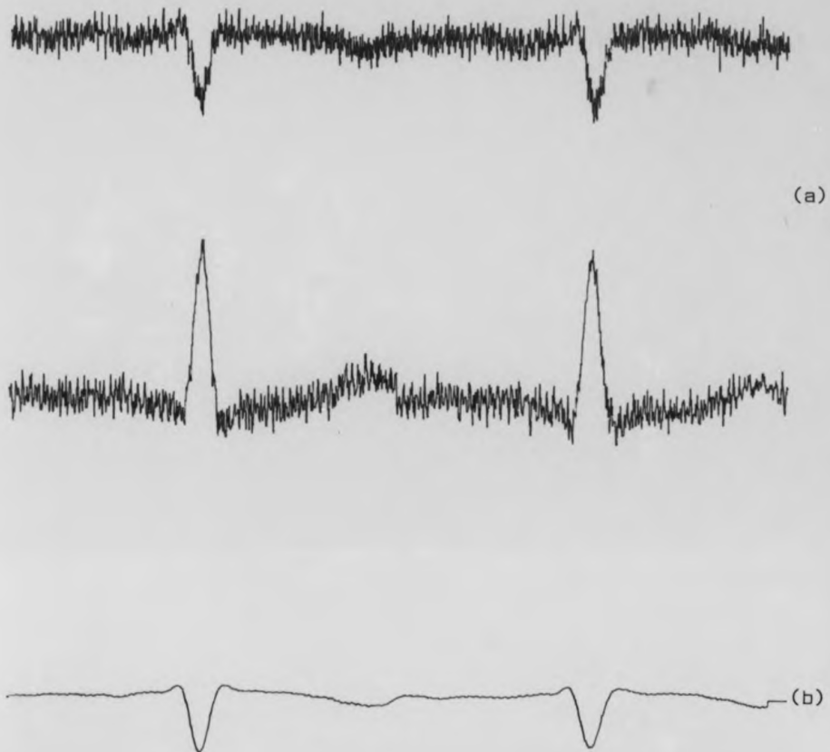
Figure 7.16 The result of applying high pass filter to remove dc baseline fluctuations and then applying the adaptive technique to remove the skeletal muscle activity, the figure above shows: (a) the two recorded channels necessary for adaptive filter to perform, the convergence factor was 0.001 and it was 64 weight coefficients (b) the result of high pass filter prior to the adaptive filter for the V_1 lead
