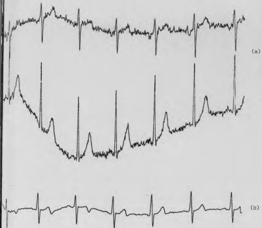
Figure 7.10 The result of applying high pass filter to remove dc and baseline fluctuations and then applying the adaptive technique to remove the skeletal muscle activity, the figure shows:
