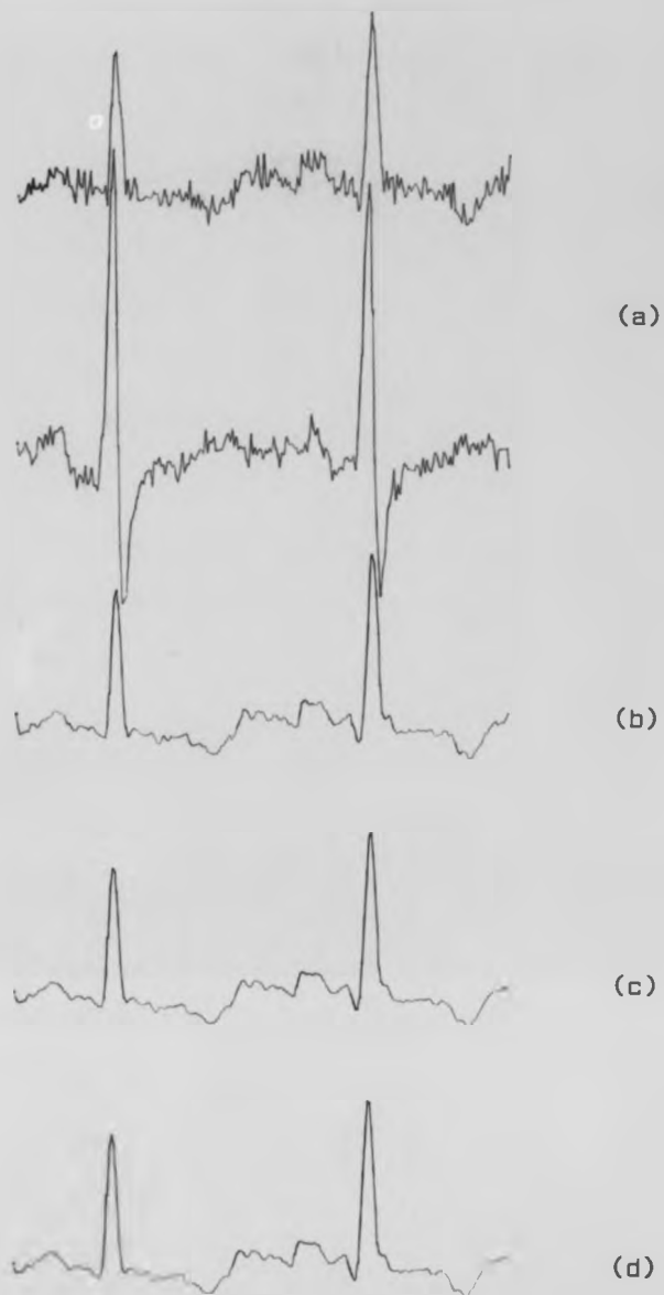
Figure 8.16 Comparison of filter outputs for the basic adaptive filter (AF), time-sequence adaptive filter (TSAF) and minimal time-sequence adaptive filter (MTSAF) using real exercise ECG. The adaptation speed \mu = 0.001 , filter order N = 64
