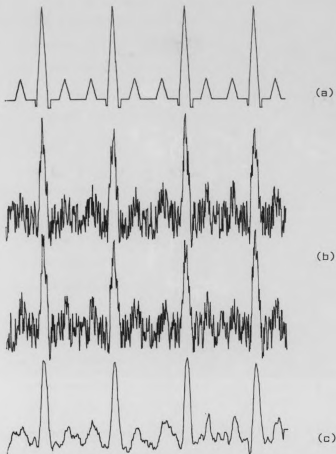
Figure 6.5 Result of applying adaptive filtering technique to simulated data (SNR = 3.47dB)
