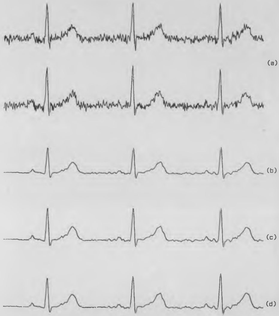
Figure 5.6 Comparison of three adaptive filters (AF, TSAF and MTSAF) using low SNR (SNR = 9dB), the figure shows: (a) the two input signal and noise (b) the result of adaptive filter (c) the result of time-sequence adaptive filter (d) the result of minimal time-sequence adaptive filter the convergence factor is 0.001.
