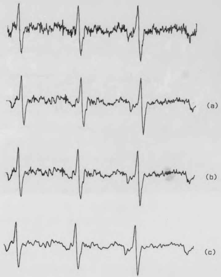
Figure 3.9 Results of applying transversal filter with different weight coefficients to exercise ECG.
