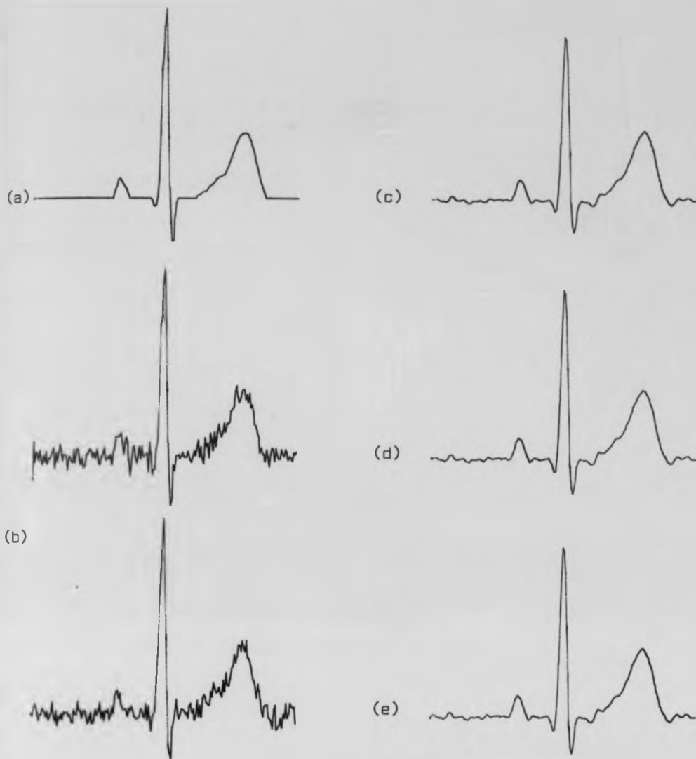
Figure 8.14 Comparison of filter outputs for the basic adaptive filter (AF), time-sequence adaptive filter (TSAF) and minimal time-sequence adaptive filter (MTSAF) using simulated data, SNR = 13.24dB, adaptation speed \mu = 0.001 , filter order N = 64
