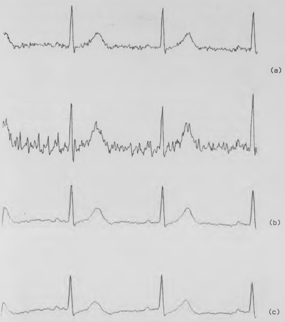
Figure 8.8 A comparison of the effect of the filter convergence factor upon adaptive filter, the filter order N = 64 . (a) the two input signals (b) convergence factor = 0.01 (c) convergence factor = 0.001
