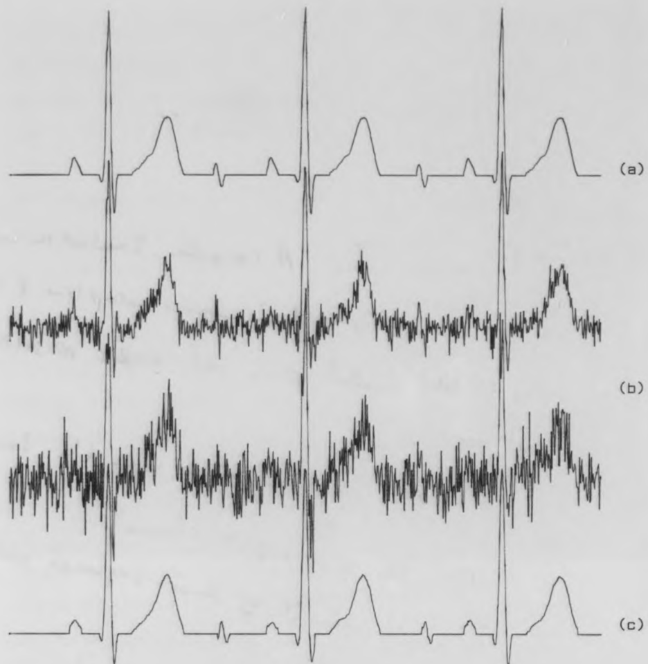
Figure 6.22 A computer simulation result of applying time-sequence adaptive filters to detect the simulated foetal ECG of SNR = 10.3dB. The figure shows:
