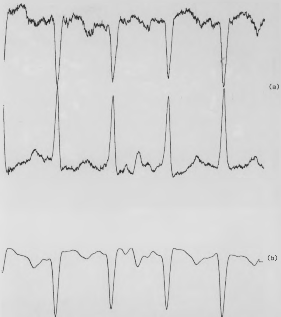
Figure 7.15 The result of applying high pass filter to remove dc baseline fluctuations and then applying the adaptive technique to remove the skeletal muscle activity, the figure shows:
