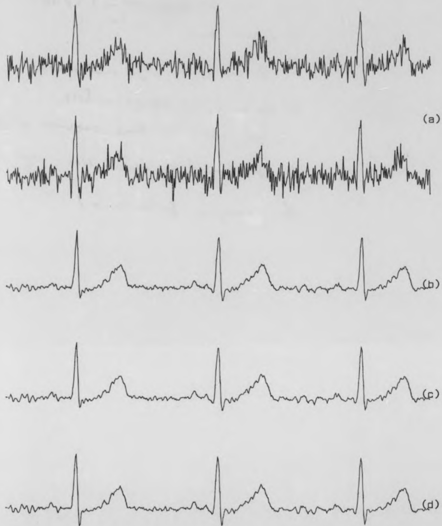
Figure 5.5 Comparison of three adaptive filters (AF, TSAF and MTSAF) using low SNR (SNR = 3.58dB), the figure shows:
