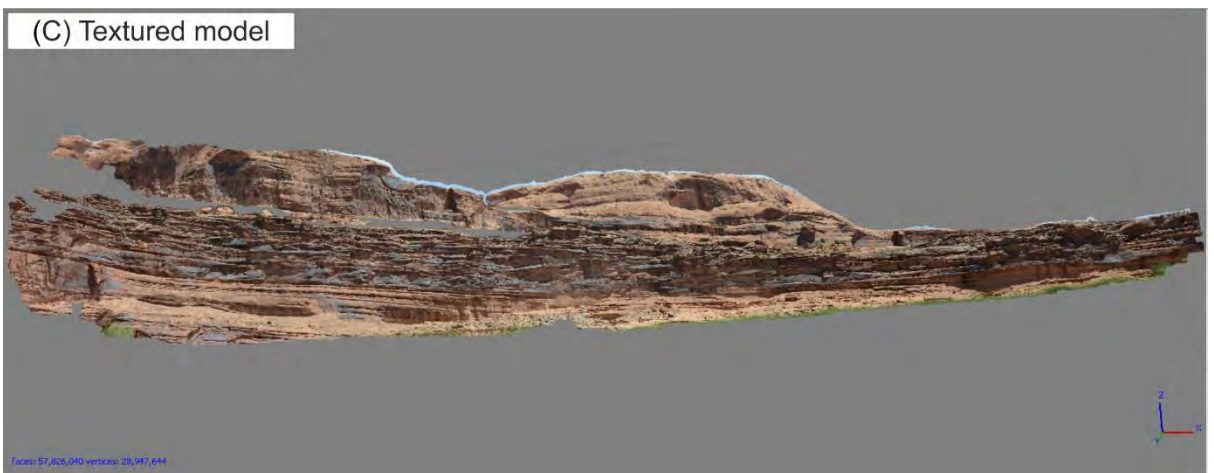
Figure 3.5. Construction of Model 1 (proximal – Lions Park) using Agisoft PhotoScan. (A) Sparse point cloud generated using SfM – 26,703 points. (B) Dense point cloud generated using MVS with pixel grid-based matching – 289,130,233 points. (C) Photo-realistic textured model.
