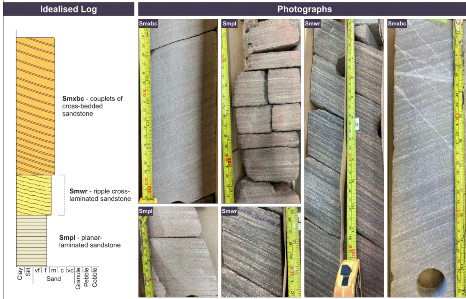
Figure 8.6. Summary panel of the aeolian dune plinth association of the Leman Sandstone with an idealised log and photographs of the internal facies.
