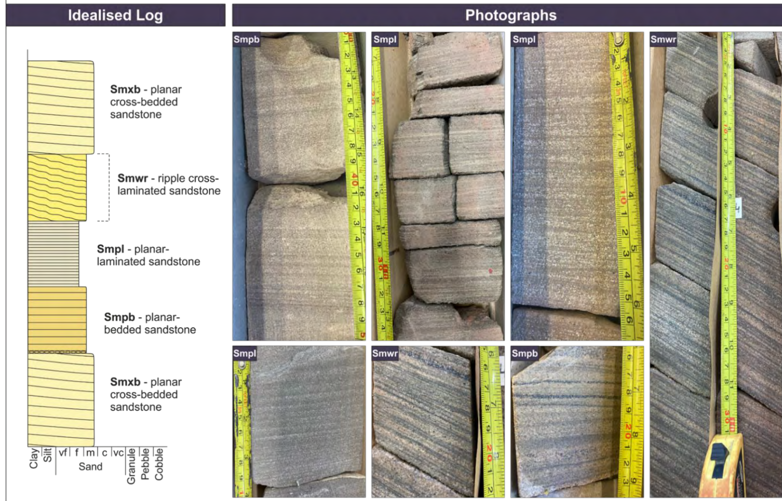
Figure 8.8. Summary panel of the aeolian dry interdune association of the Lemna Sandstone with an idealised log and photographs of the internal facies.
