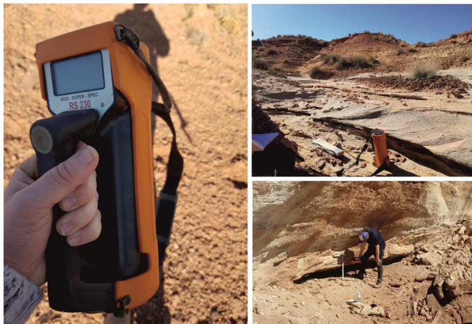
Figure 5.3- Positions of the spectrometer were chosen based on the most effective angle for measurement as outlined by Svendsen & Hartley, 2001.
