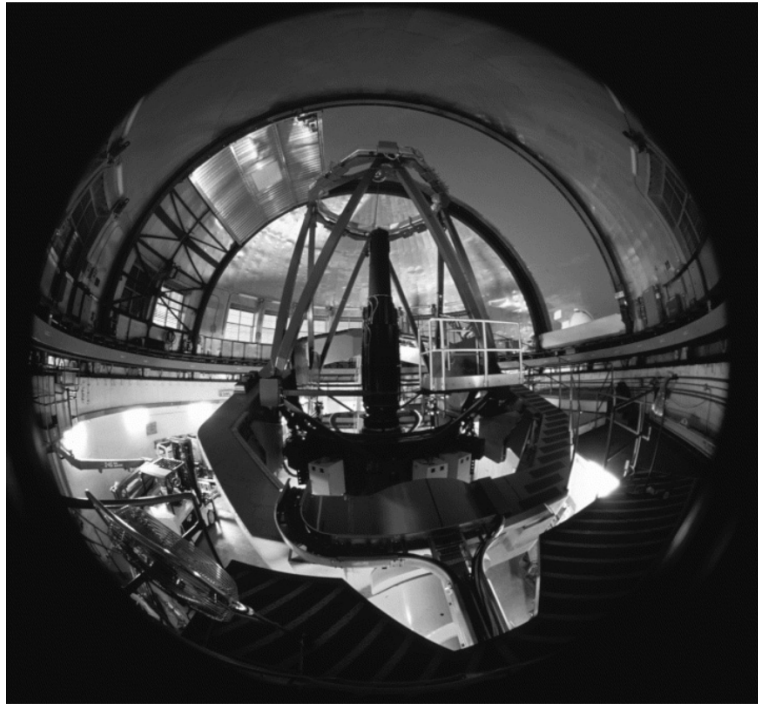
Figure 3.1: A photograph of WFCAM mounted on UKIRT, reproduced from fig. 1 of Casali et al. (2007). The telescope is pointed towards the zenith and the camera is the dark cylindrical element rising from the centre of the primary mirror.
