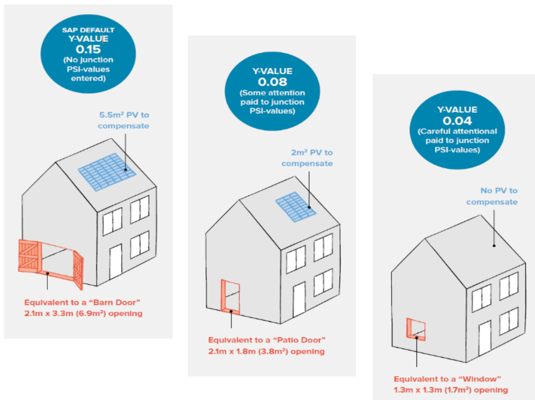
Figure 4 The impact of thermal bridges represented by different sizes of doors
