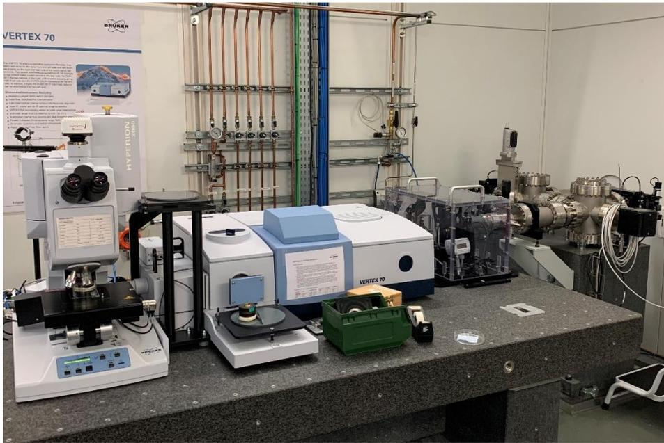
*Figure 8 Bruker Vertex 70 spectrometer with Hyperion 3000 microscope at MIRAS beamline in ALBA synchrotron.*
