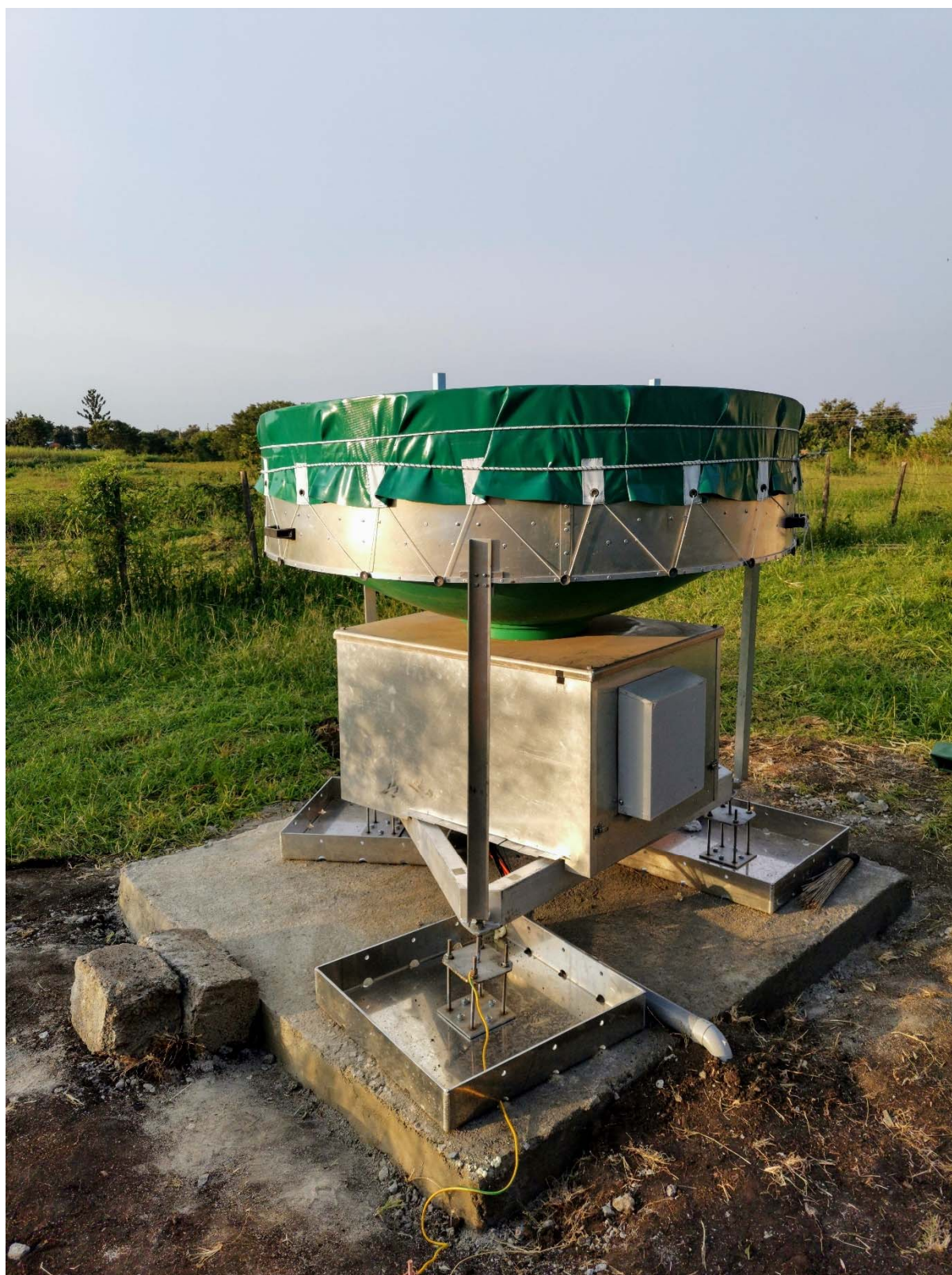
Figure 2: The vertical looking radar installed at ICIPE Mbita, on the shores of Lake Victoria.
