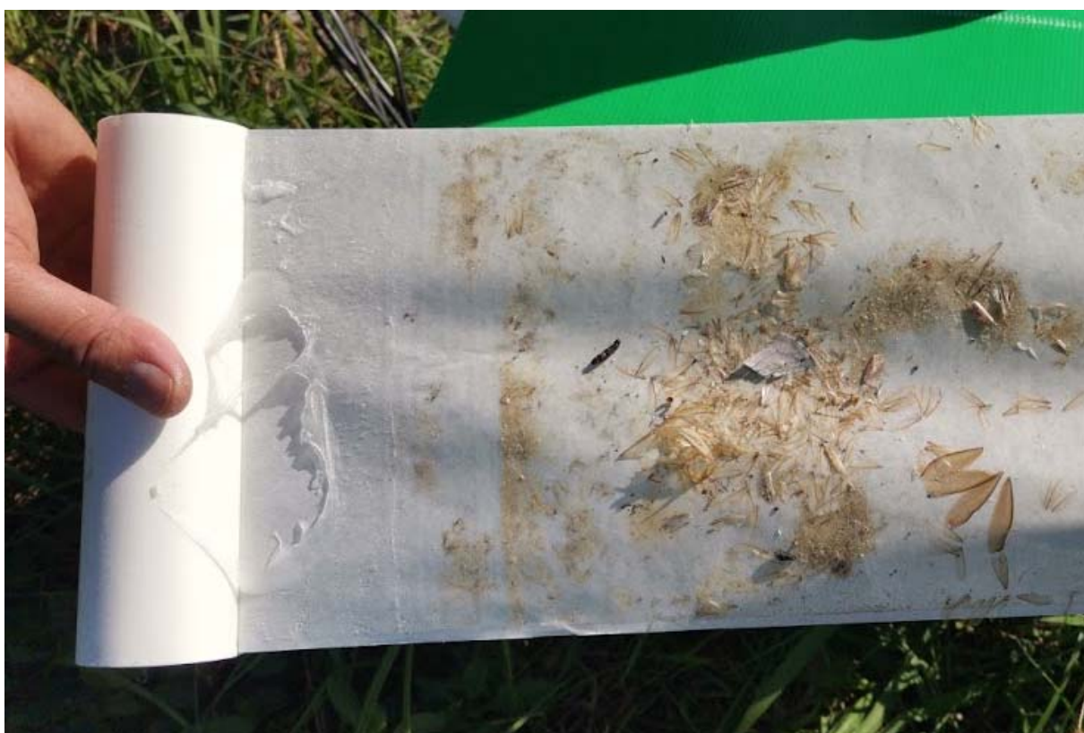
Figure 5: Defective sticky roll taken from the trap in Mbita. A combination of high temperatures and humidity caused the glue on several of the sticky rolls to degrade. The motor could not turn to replace the upper surface, which was no longer adhesive, affecting the operation of the digital pheromone traps.
