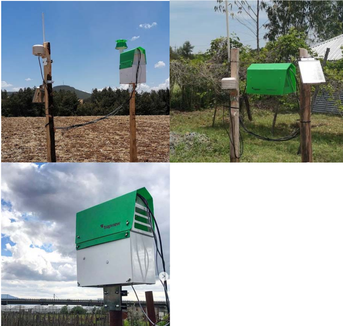
Figure 6: Examples of a digital funnel trap (top left), digital delta trap (top right) and digital slit trap (bottom left (not site-specific photographs)). The delta trap and slit trap were placed within a 25m of the funnel trap at the KALRO site in Embu in June 2019. The slit trap was only operational for a period of five months following theft of the solar panel, but we continued to operate the delta trap until the project close in March 2020.
