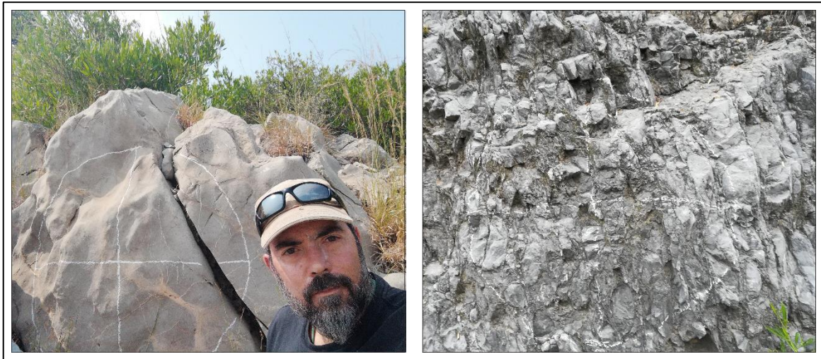
Figure 3.17: Examples of measurement circles chalked on the rock-mass which can be highly fractured. The chalk circle is not clear in the right-hand image due to the high degree of fracturing. To compensate for this, circles of the appropriate size are drawn during the compositing of the photographs of a measurement circle.
