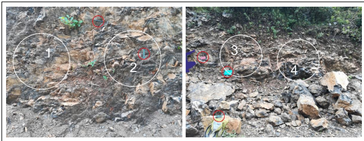
Figure 4.167: Positions of measurement circles on the south-eastern sidewall of the road at site 4. Pens and notebooks are circled in red for scale. View is along strike.
