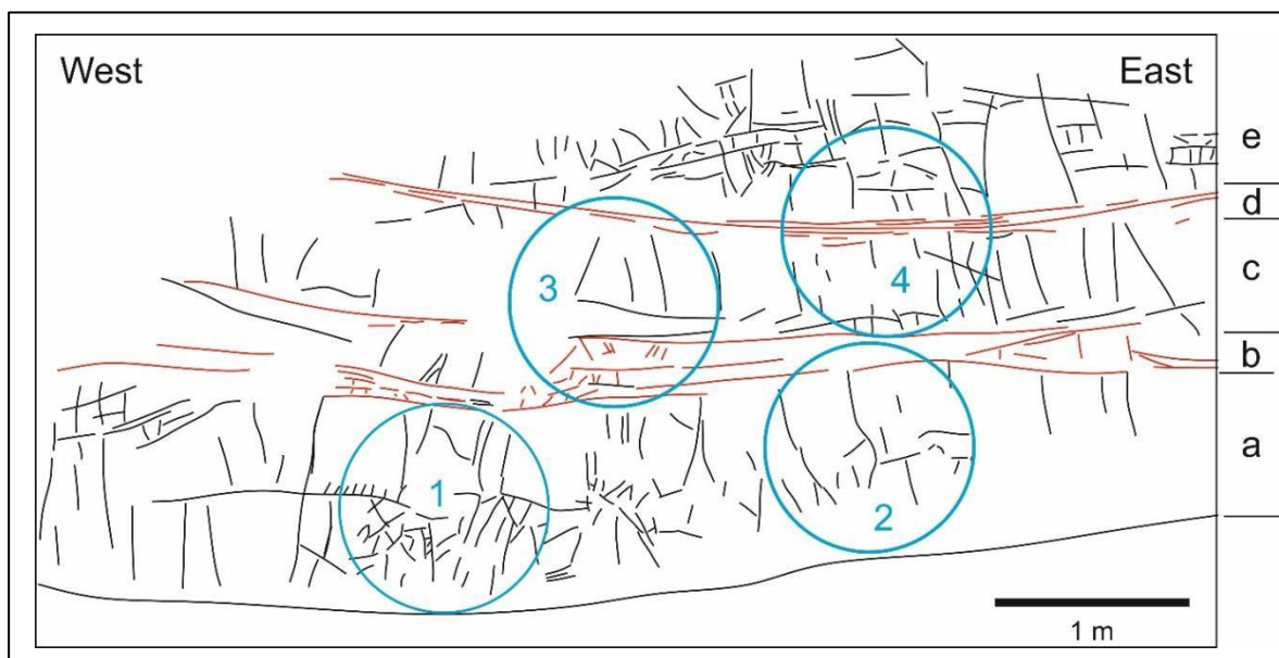
Figure 4.63: Line drawing of the fracture patterns at site 3 derived from Figure 4.62 . Five layers are recognised with the thicker layers (a, c, and e) being dominated by near-vertical fractures (shown in black). In contrast, the thinner layers (b, and d) contain mainly horizontal fractures (shown in red). The positions of measurement circles are also indicated in blue.
