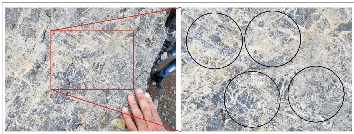
Figure 4.85: View of earlier generations of fractures exposed on a late-stage fracture surface (see Figure 3.24). The zoomed in view (right) shows the distribution of 5 cm wide measurement circles.
