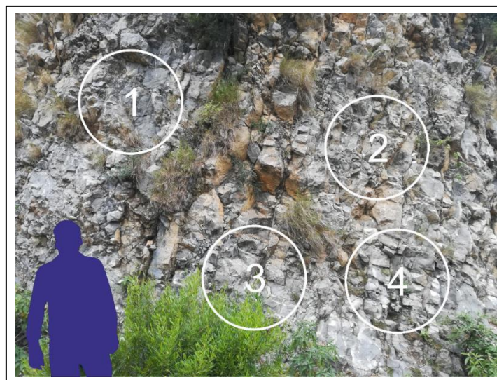
Figure 4.124: Distribution of measurement circles on the western sidewall of the road cutting at site 4. Geologist in blue.
