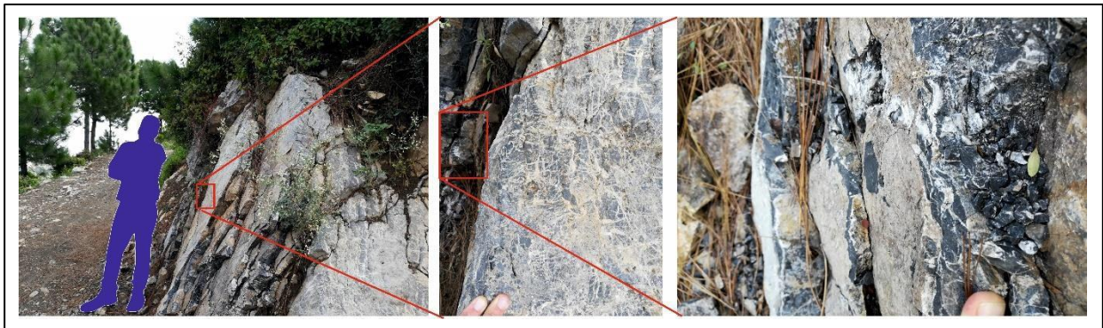
Figure 4.83: Outcrop at site 7 – dark grey Kawagarh Formation limestone with small millimetre-sized calcite fractures throughout. Strongly developed layering related to the folding and overturning of the anticline axis at this site (Figure.4.49) is super-imposed on these fractures. Geologist in blue.
