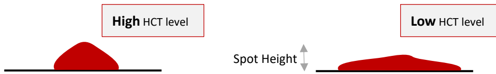
Figure 4-1. Figure showing the differences in blood spot depending on the HCT levels within a person.
