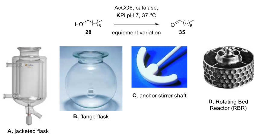
Scheme 43 - Bioprocess of octanol 28 (100 mg, 0.8 mmol, 1.0 equiv.) with equipment variation, AcCO 6 form and aminomethyl resin 66 . Reagents and conditions: singlate, 1.7 mM octanol 28 (100 mg, 0.8 mmol, 1.0 equiv.), AcCO 6 (immobilised or CFE), 0.04 mg.mL -1 catalase (CFE), aminomethyl resin 67 , 100 mM KPi buffer (pH 7.0), 37 °C, 200 rpm, overnight. Source image: Radleys® , Sigma-Aldrich® , Spinchem® .
