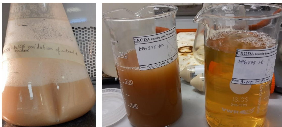
Image 1 – Biotransformation of octanol 28 (500 mg) with AcCO6 CFE after 24 h reaction (left), which solution was separated in equal volume and quenched with 5.0 M NaOH 83 (middle) or quenched with 5.0 M HCl 84 (right)
