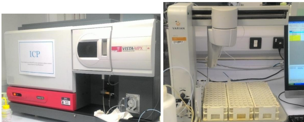
Figure 2.5: ICP-OES on the left and autosampler on the right hand side.
