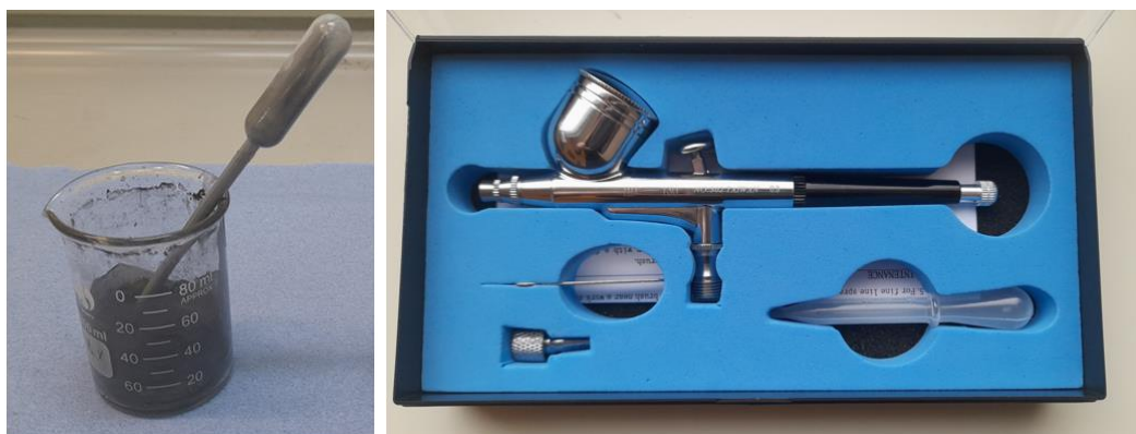
Figure 4.2: (left) Ink, (right) airbrush used to deposit ink on the substrate.
