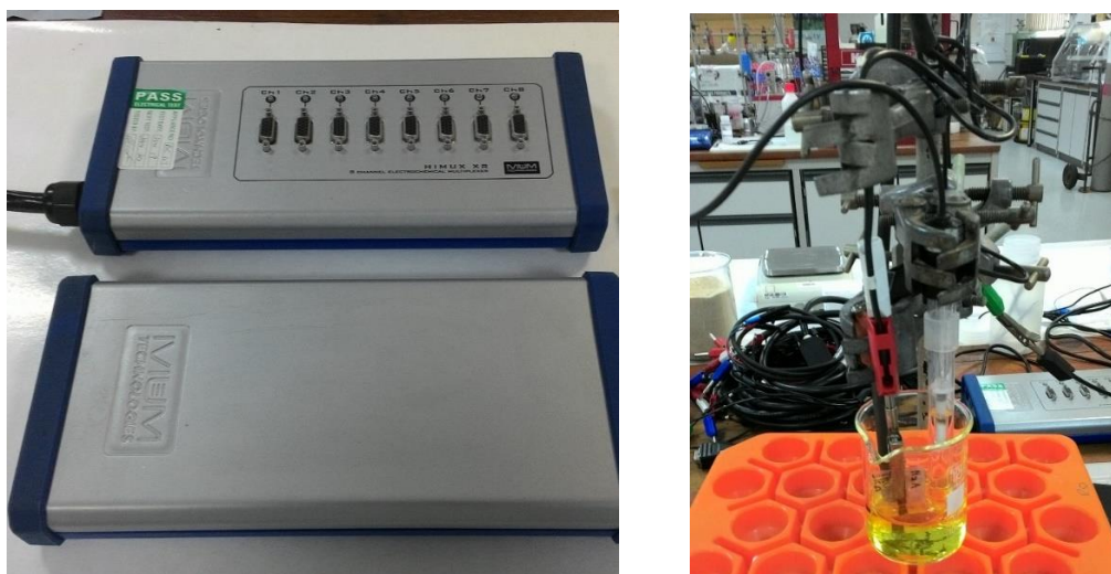
Figure 4.3: (left) Ivium potentiostat model CompactStat.h (bottom), multiplexer (top). (right) Setup adopted for EIS experiment.
