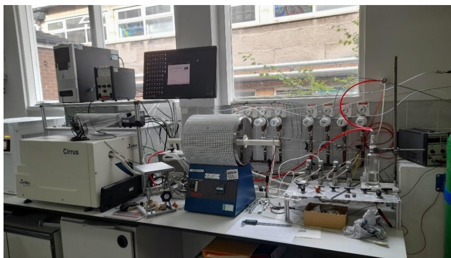
Figure 2.11: Quadrupole mass-spectrometer MKS Cirrus with furnace and gas line.
