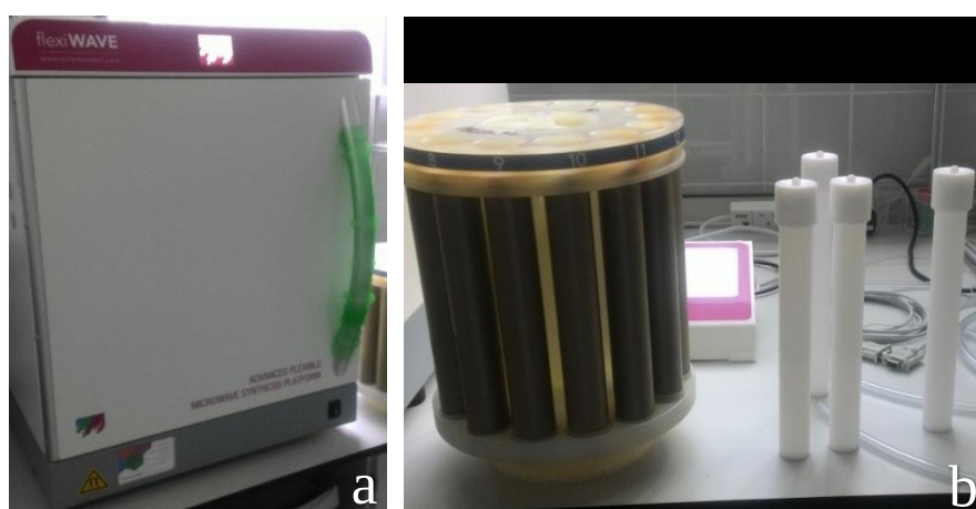
Figure 2.4: (a) Microwave and (b) carousel with vessels.
