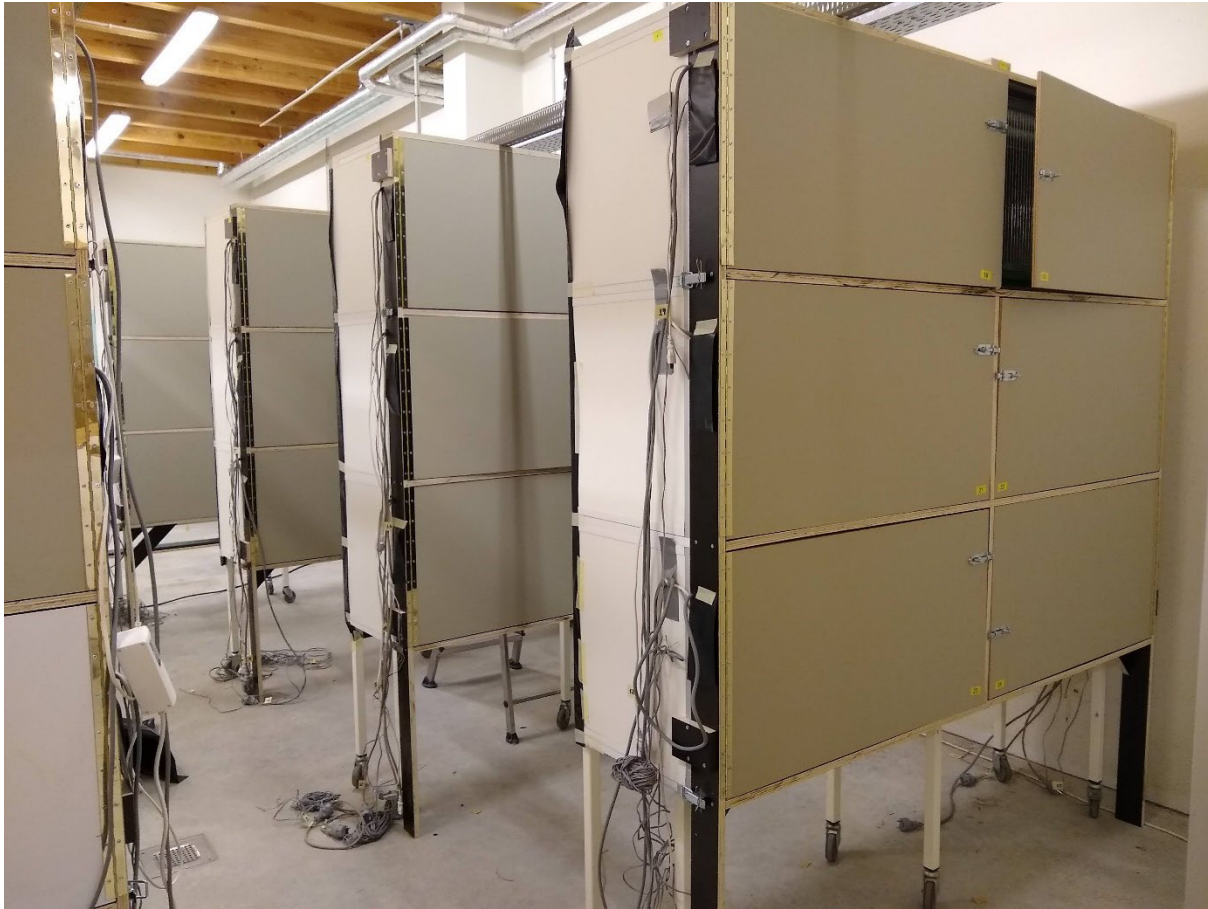
Figure S1_1: Photo of the experimental set-up for measuring activity rhythms. We had groups of 6 individual cages with a metal front in stand-alone plywood racks. Cages were separated from one another by wood panels that surrounded them except for the front side. These panels prevented birds from seeing any of their neighbours. The front of the cages was covered by a wooden door that could be opened for feeding and caretaking. Photo by Barbara M. Tomotani.
