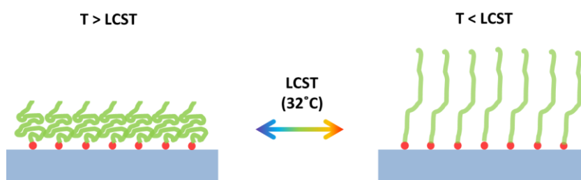
Figure 5.1 - The lower critical solution temperature (LCST). At either end of the LCST the morphology of the NIPAAm polymer chains change.
