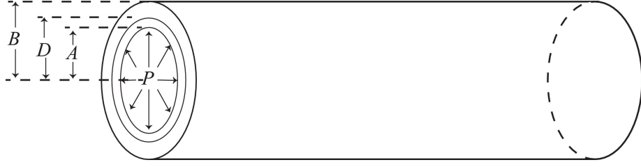
Figure 4.11: A bilayer tube with inner radius A and outer radius B under internal pressure P and axial load F .
