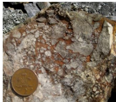
Figure 8. Calcite-cemented sandstone breccia. The cementing calcite contains a few tiny grains of chalcopryite, though none is visible in this photograph. Photo. B. Young
