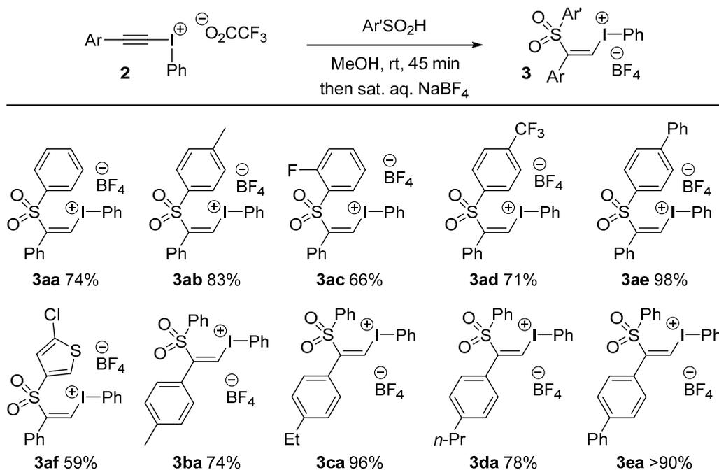
**Scheme 3.** Preparation of alkenyl(phenyl)iodonium tetrafluoroborates **3**.
