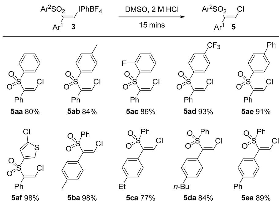
**Scheme 5.** One-pot conversion of iodonium salts **3** to vinyl chlorides **5**.
