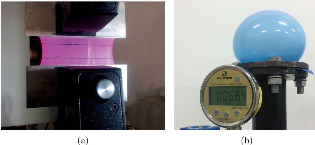
Figure 6: Final stages of (a) pure shear and (b) biaxial extension.
