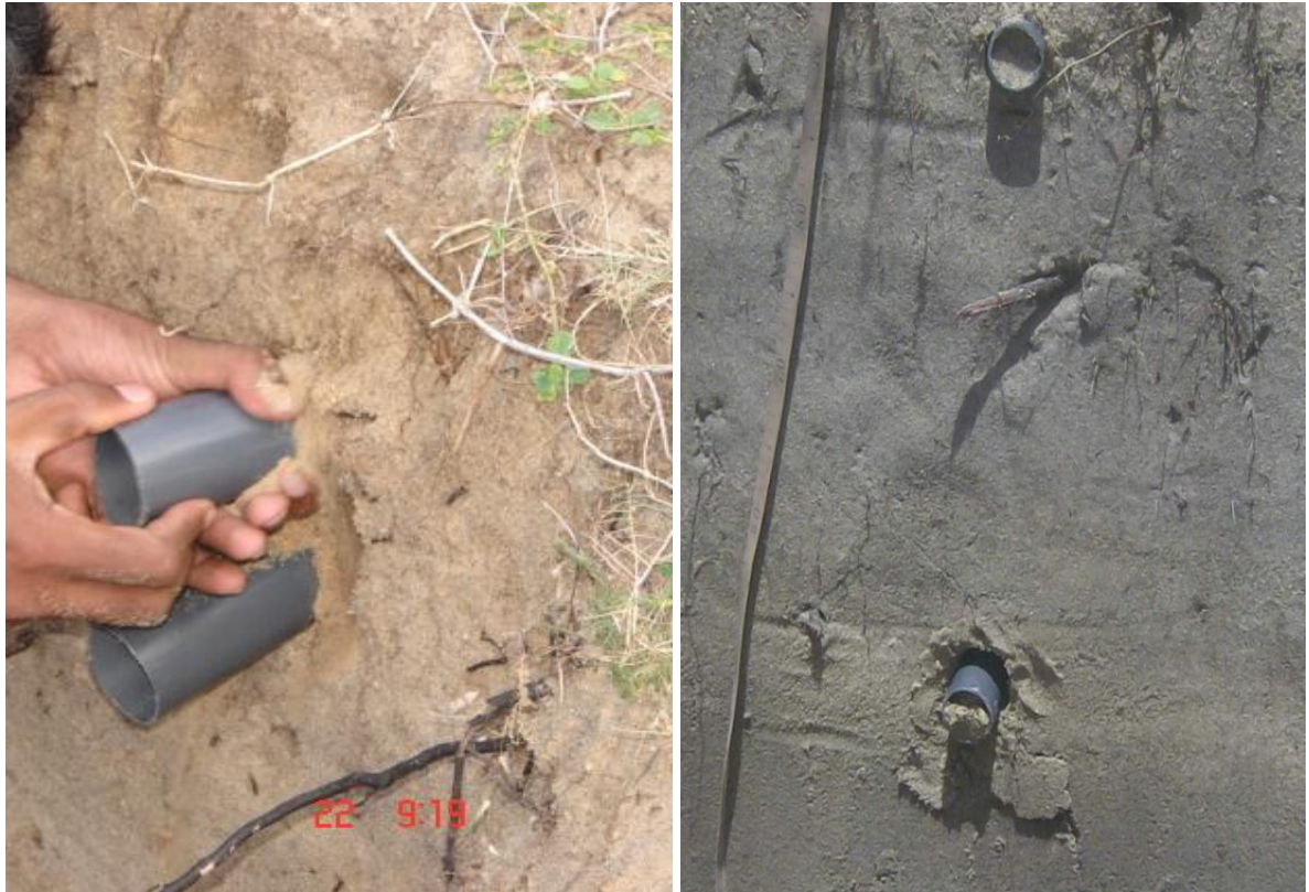
Figure 3.23: Sediment sampling for OSL analysis.
