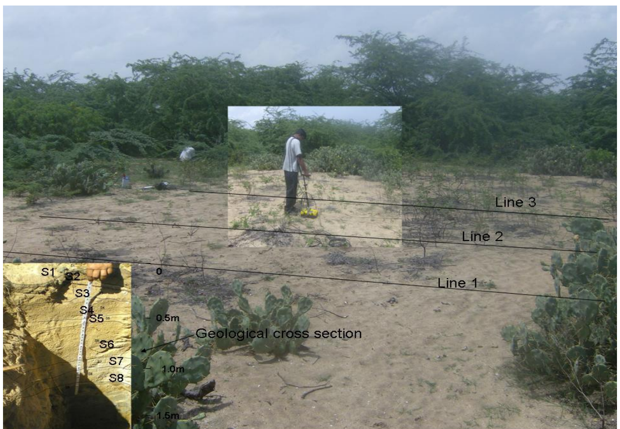
Figure 6.3 GPR survey Line 1, 2 and 3 at site 2- Hambantota, south-east coast of Sri Lanka.
