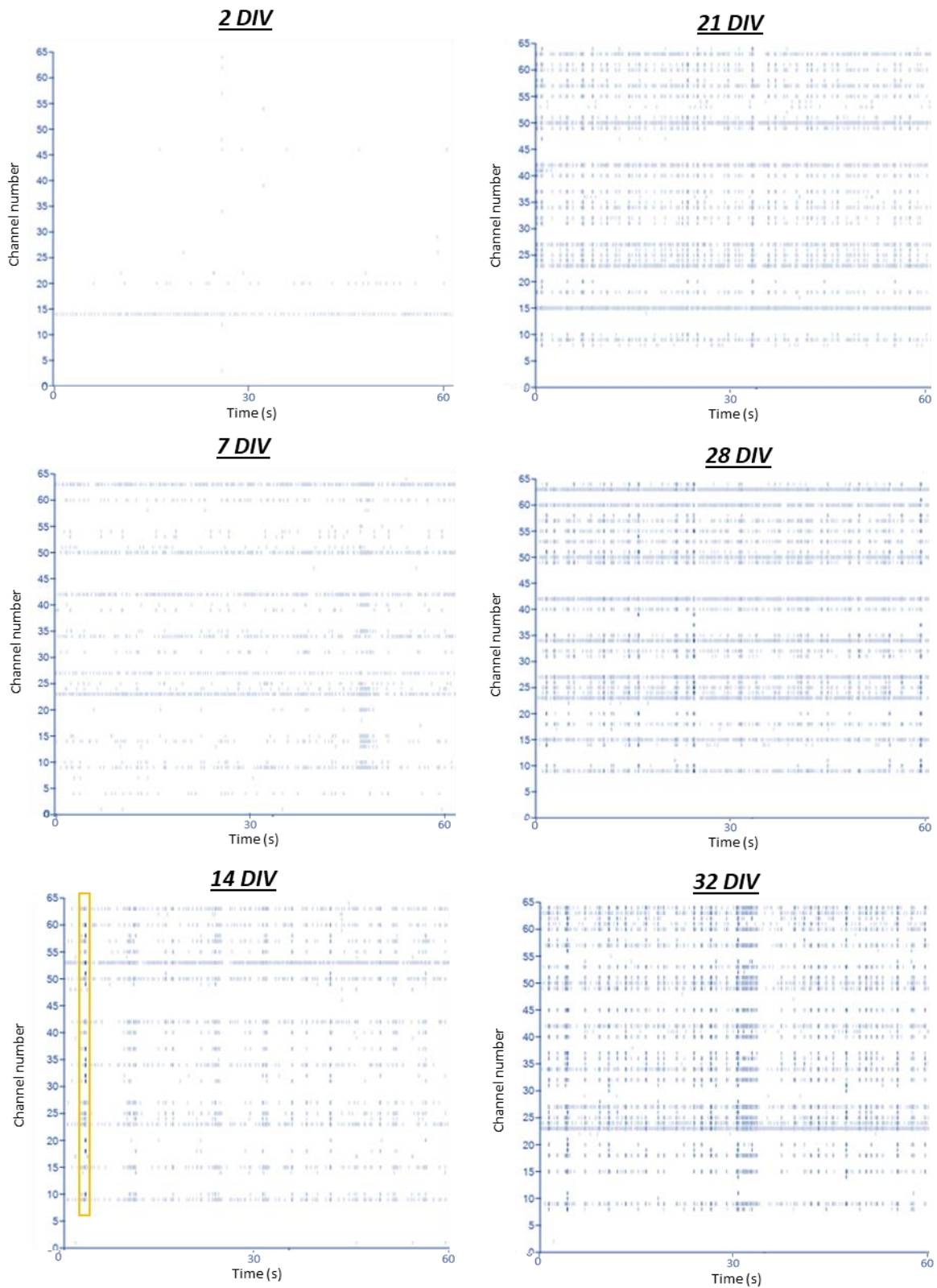
Figure 5.7. Array-wide 60 second raster plots from the same culture over 32 DIV. These spike detection plots show an increase in spontaneous spike frequency, bursting and synchronicity recorded from 64 electrodes. Yellow box indicates one of the many synchronised bursting events.
