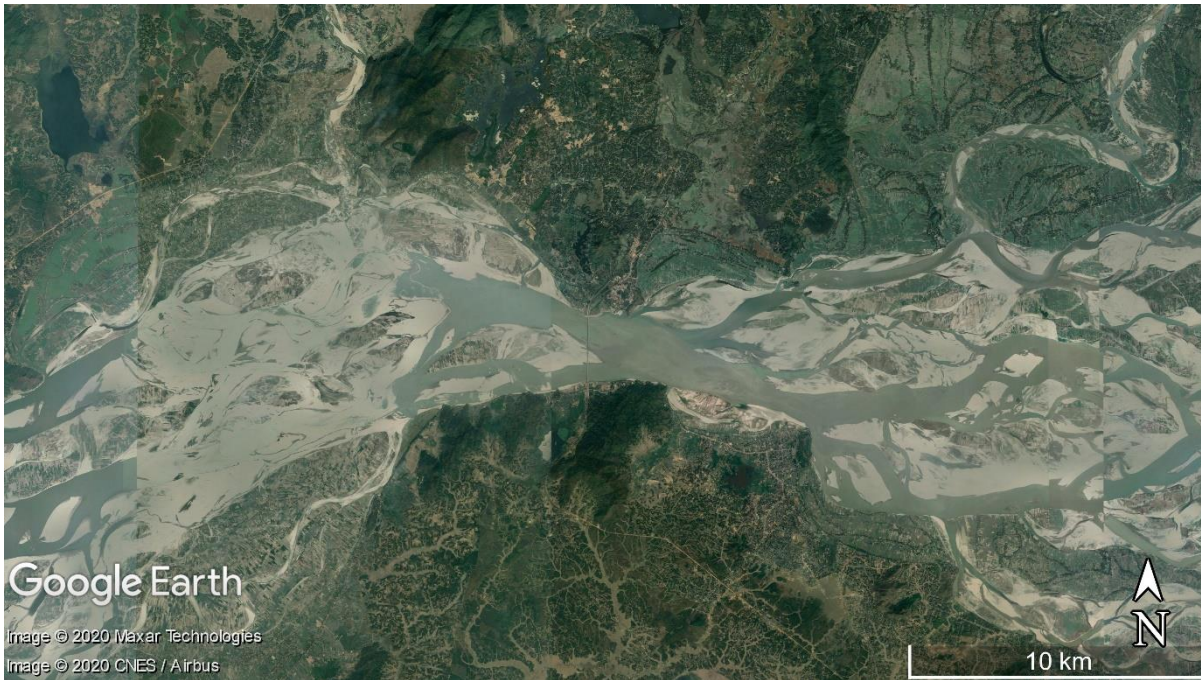
Figure 6.3 – Jamuna River, northern India, showing a confined morphology with submerged unit bars and a large amount of sediment deposited distal of the confinement.
